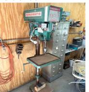
· Powermatic Heavy Duty Drill Press, Model 1150A, 3/4HP, 110-V, Single Phase
