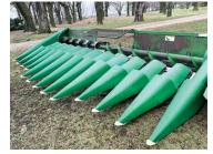
John Deere 843 Head, Converted to 12 Row 20" Spacings, Poly Snoots, **Dual PTO**
