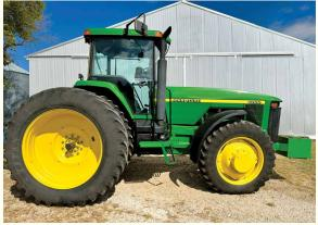
• 1998 John Deere 8200 MFWD Tractor, 6159 Actual Hours, John Deere ATU 200 Steering Unit, 4 Hydraulics, 3pt with Quick Hitch, 540/1000PTO, Hammer Strap Hitch, (4) 205 KG Inside Rear Wheel Weights, 480/80R46 Rear Duals, 380/85R34 Front Tires with Fenders, Rock Box, Clean Tractor, Ag Diesel Solutions Chip, SN: RW8200P020417
