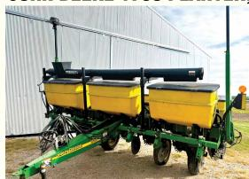
• 2007 John Deere 1750 MaxEmerge XP Planter, Vacuum, 6 Row 30", Dawn Row Cleaners, Markers, Dry Fertilizer with Cross Auger, Fertilizer Box Extensions, Seed Box Extension, Computer-Trak 350 Monitor, Corn & Bean Plates, Fertilizer Disc, AMVAC Smart Box Insecticide Boxes, New Drive Chains, New Disc Openers with 250 acres on them, SN: A01750R725159, very clean
