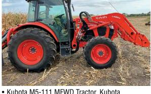
Kubota M5-111 MFWD Tractor, Kubota LA1854 Hydraulic Loader w/Joystick, 1360 One Owner Hours, 24 Speed w/Two Speed Power Shift Transmission, Left Hand Reverser, 460/85R30 Tires, 3pt., 540/1000PTO, Aux. Loader Hydraulics, 84" Bucket, SN: KBUM4EDCLL8M64365
