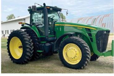
2009 John Deere 8330 Tractor MFD Powershift Trans, 3500 hrs, 4 Hyd. Remotes, 540/1000 PTO, 60 GPM hyd. pump 480/80R46" Tires & Duals, HID Lighting Front & Rear, Buddy Seat, Autotrac Ready, JD Active Seat
