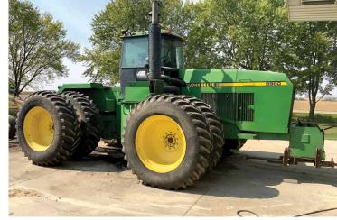
1990 John Deere 8960 Tractor, 8866 hrs 20.8x42" Tires and Duals, 3 Hyds, 24 speed Trans, Weights, Front Rock Box, Sells with JD ATU Auto Steering Kit with Globe
