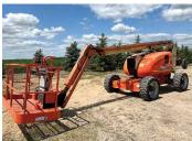
\*\*\* 2011 JLG 600 AT Manlift, 3719 Hours, 60' Max Height, 39' Max Horizontal Reach, 500 Lb. Capacity, 49hp Deutz Diesel, 3'x8' Man Basket, Ground Controls, Excellent Condition
