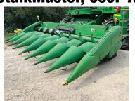
\*\*\* 2010 John Deere 608C StalkMaster Corn Head, 8 Row 30", Chopping Head, Stubble Lights, Hyd. Deck Plates, Contour Master, Row Sense Updated Gear Boxes In 2014 Many New Parts In Last 2 Years. 8 Row Stalk Stomper Bar. SN: H0608CCJA0735768
