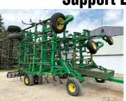
\*\*\* John Deere 2210 Field Cultivator, 50.5', 2 Bar Coil Tine Harrow, Rolling Basket, Floating Hitch, 200lb Shanks, 7" Knock-On Sweeps, 6" Spacing, New Transport Tires, One Owner, SN: 1N02220XAE0755849
