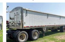
\*\*\* 2009 Wilson Pacesetter DWH-500 Hopper Grain Trailer, 34'x66"96", 24.5 Tires, 4500HD Electric Tarp with Remote
