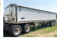
\*\*\* 2019 Wilson Pacesetter DWH-600 Hopper Grain Trailer, 34'x66"96", ABS, 24.5 Tires, 4500HD Electric Tarp with Remote
