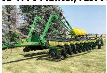
\*\*\* John Deere 1770 Conservation Planter, 24 Row 30", Liquid Fert., 3 Bushel Poly Boxes, Row Cleaner, 500 Gallon Poly Tank, Row Shut Offs, John Deere Computer Trak 350 Monitor, Planter was Completely Rebuilt, Excellent Condition, SN A01770B705177
