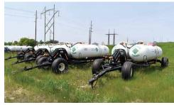
(20) Dalton 1450 Gallon NH3 Field Tanks, with Dalton WN-1600 Running Gears, (6) Have Adjustable Axles, Most have Brakes
