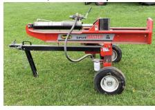
Like New SpeeCo Log Splitter, 22 Ton, Trailer Style, B/S Power Unit
