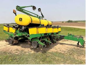
\*\*\*John Deere 1760 Conservation MaxEmerge Plus Planter, 12 Row 30", Liquid Fertilizer (2) 225 Gallon Liquid Tanks, Markers, Row Cleaners, Front Fold, Vacuum, Quick Fill Valves, Spike Closing Wheels, Insect, Seed Firmers, Precision Corn Disc And Regular Bean Disc, JD 250 Monitor, In-Furrow Fertilizer. SN: H1760F675403
