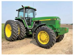
\*\*\*1992 John Deere 4560 MFWD Tractor, 7872 Actual Hours, 2000 Hours On JD Overhaul W/Paperwork, 15 Speed Power Shift, 480/80R42 Michelin Duals At 95%, 580/85R30 Michelin Front Tires At 95%, Front Fenders, 14 Front Suitcase Weights, 3pt With Quick Hitch, 3 Hydraulics, Big 1000PTO, Extra Lights, Cold A/C, SN: RW4560P001258, Very Clean
